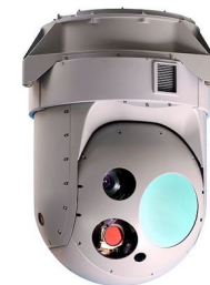
Example EO/IR Sensor
